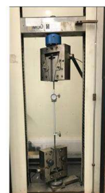
Grips rotated to shorten & lengthen the rope lay length.
